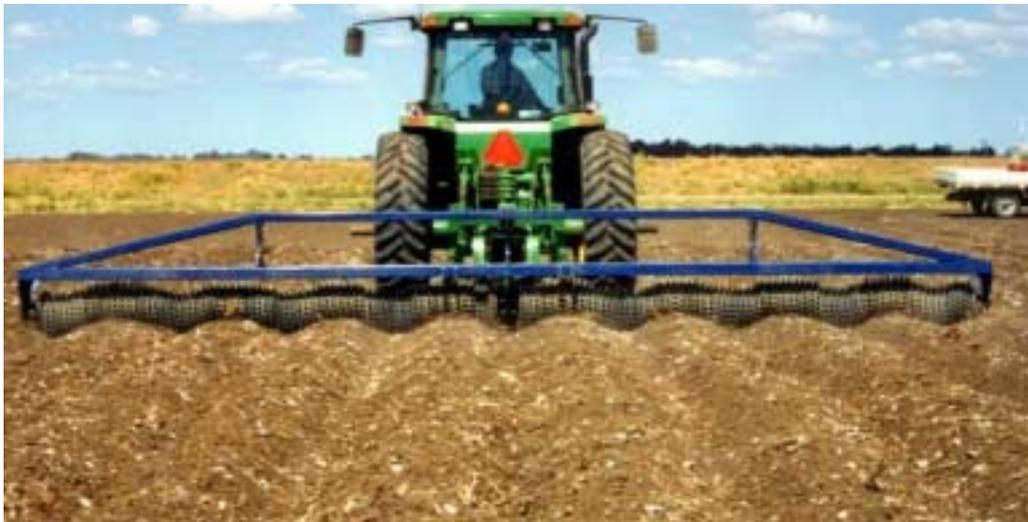
**Figure 3.4:** The Contour Following Ability is Ideal for Raised Beds.
